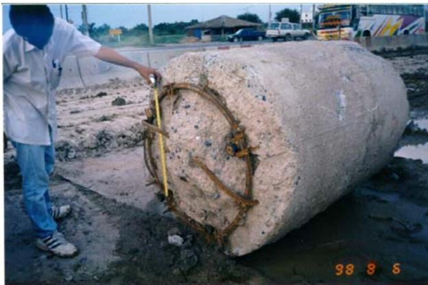
Figure 7. Typical model pile used to determine manchette breaking mechanism.
