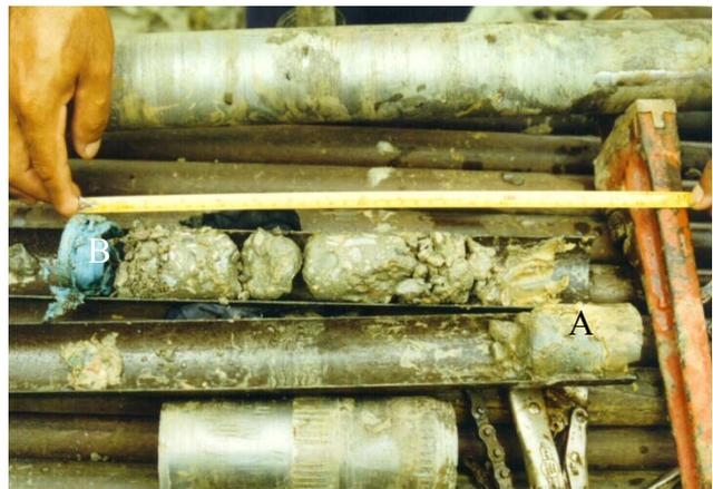
A: Grout core, B: PVC-casing bottom cap.
